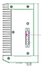
AC Power — Connect the AC power supply to the Sensor by inserting the 12-36V DC 6pin Phoenix Contact connector into the side of the Sensor unit and tightening the embedded screws at the top and bottom of the connector.
