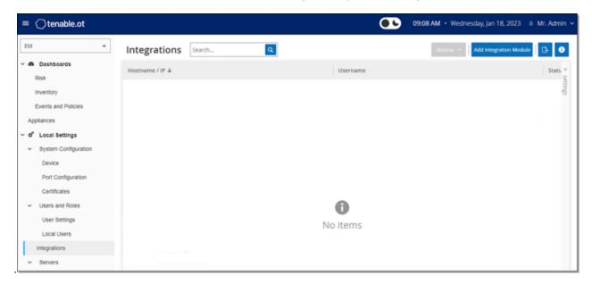
**Note**: To integrate the platforms, OT Security must be able to reach Tenable Security Center and/or Tenable Vulnerability Management via port 443. Tenable recommends that you create a specific user on Tenable Security Center and/or Tenable Vulnerability Management to be used as the integration user to OT Security.
