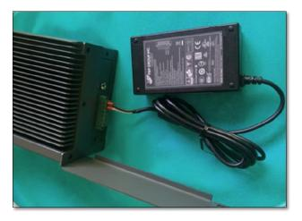
Then, insert the AC power supply cable (provided) into the power supply unit, and plug the other end into an AC outlet.
