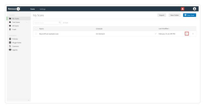
16. Once the scan is complete, select the completed scan and look for the corresponding message - *OS Identification and Installed Software Enumeration over SSH: 97993.* This validates that authentication was successful.
